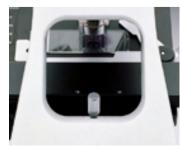
there is no chance of the objective accidentally touching the slide and damaging either the specimen or the objective itself.
