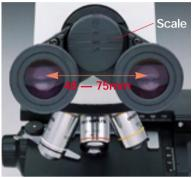
adjustment and diopter setting. High eyepoint design eyepieces with F.N.18 can be used comfortably without removing eyeglasses.
