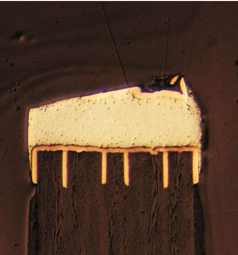
Multilayer circuit board, poor contact due to crack, original magnifications 37:1 and 600:1 (below)
