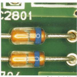
Diode on the circuit board
