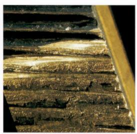
Surface of the rack after resistance test
