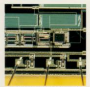
Wire bonding section on the AF sensor
