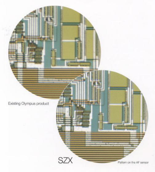
Combining the DFPLAPO1 × PF for the SZX12 with a SZX-AL20 × auxiliary objective sets another new standard, this time in resolution\*: 800 lines/mm.
