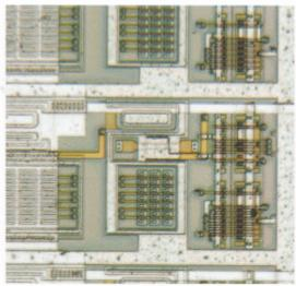
Pattern on the Charge Modulation Device ( CMD )
