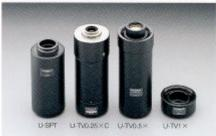
parfocal adjusting, combined with a I/3" video camera, gives an image inscribed within the observation field These adapters can be attached to the trinocular head SZX-TR30 and the photo adapter SZX-PHA directly.
